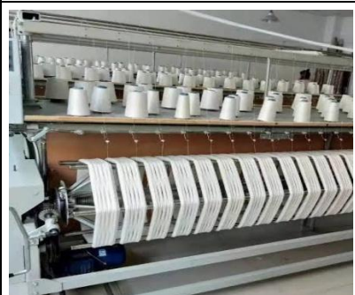
Machinery Name: Reeling machine
